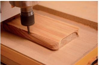
The codes are then transferred to the CNC machine, which carves the cases one-by-one out of pieces of wood. "Cell phone cases are a good use for leftover bits and pieces of wood," Shin-Min Kang notes. "What's more, even a piece of seemingly defective wood holds a great appeal to consumers because of its unique texture and fragrance."
